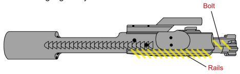
Apply CLP to the front rails on both sides of the bolt carrier and to the bolt where is it highlighted yellow.
